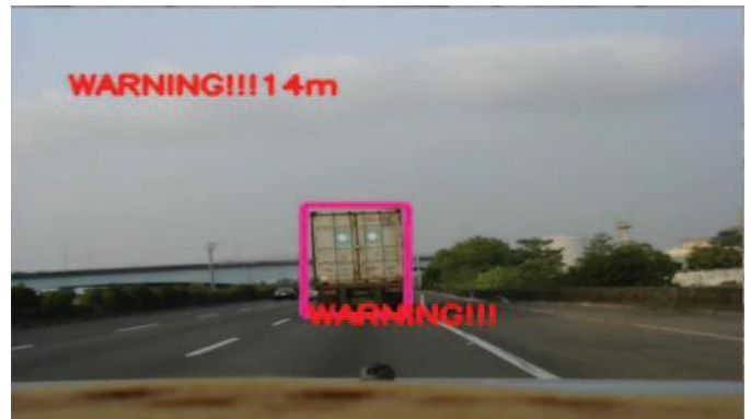
Fig -8: dangerous stated object detected
