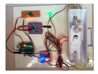
Upon rotation, the servo motor expels the designated tablet through the inclined pathway, directing it smoothly into the tray without spillage. The dispensation process is indicated by LED and buzzer alerts, providing visual and auditory confirmation of successful medication delivery. The presence of the dispensed pills in the tray is continuously monitored using an IR sensor, ensuring accurate tracking and management of medication intake.
