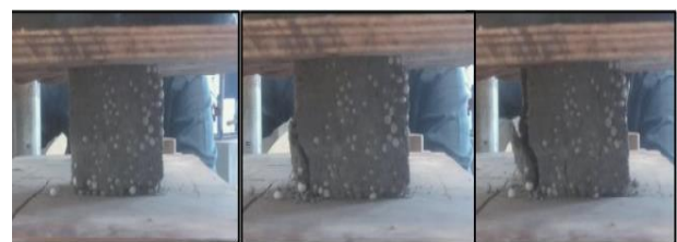
Fig -9: Failure Pattern of Specimen
