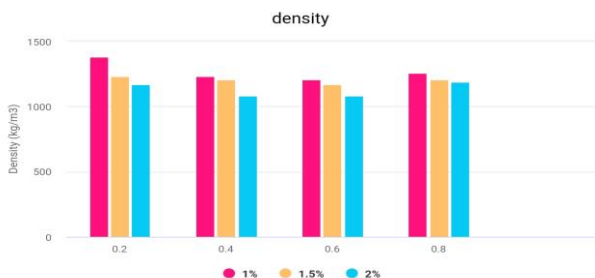
Fig -5: Effect of mix ratios on density of specimen
