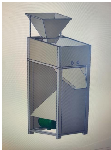
Fig-5: 3D Model of Arecanut Dehusker Machine
