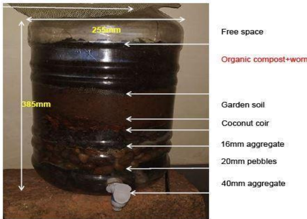
Fig-2: Experimental setup of a vermifilter
