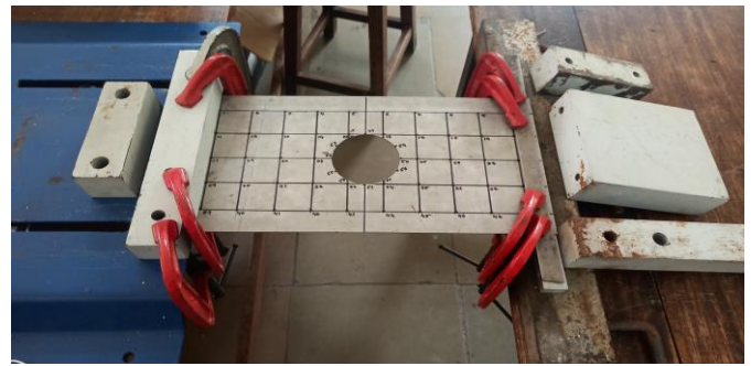
Fig 3: Plate setup for Fix-Fix test condition
