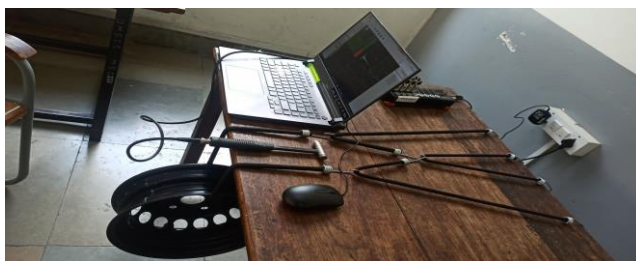
Fig. 30: Free-Free Condition setup for Rim EMA
