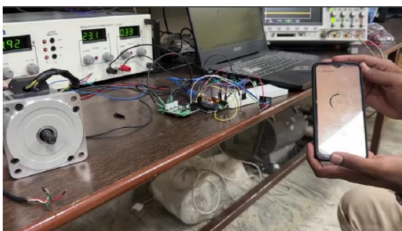
Fig -5: Demonstration of Speed Control using Blynk IoT Mobile Application
