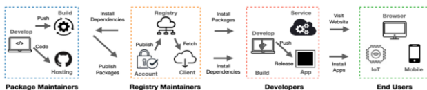
Fig. 1. Various stakeholders and their relationships in the modern OSS supply chain. Developers adopt ready to-use OSS packages for their web apps/services by installing them from Package Managers (a.k.a. Registries) into their own development environment. Package Maintainers, who may be different from the original package author, provide feature updates and security bug fixes.
