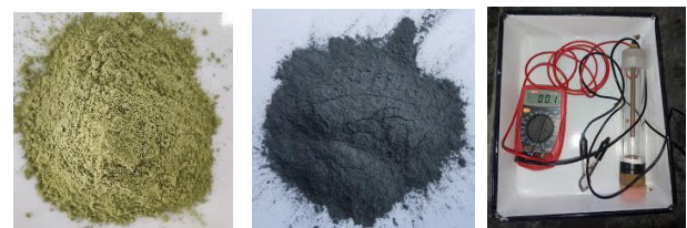
Fig -1: Neem powder (green), Zinc powder (grey) and Half-cell Potentiometer instrument
