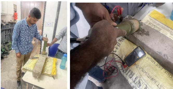
Fig -4: Testing of specimens with Half-cell potentiometer.
