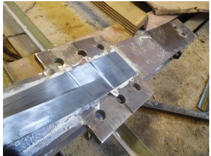
Fig -4: Typical CFRP rupture in tested beams
