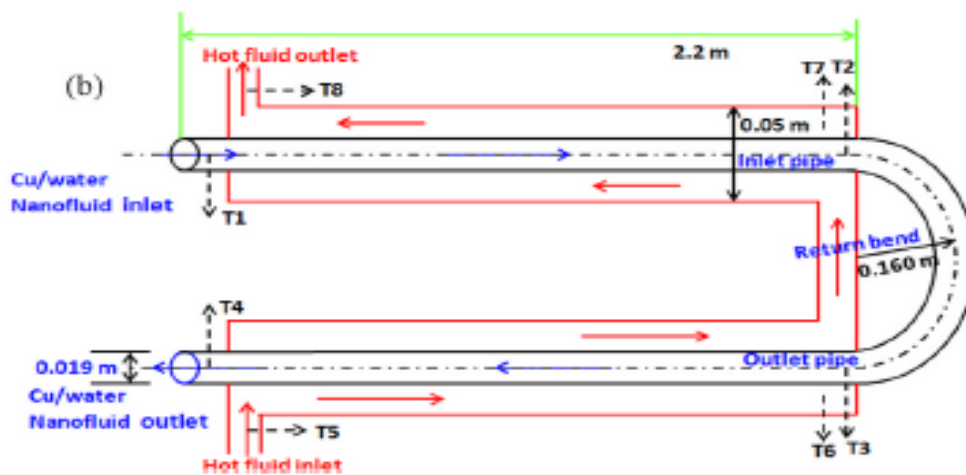
Fig. 2.2 Experimental test facility line diagram [2].
