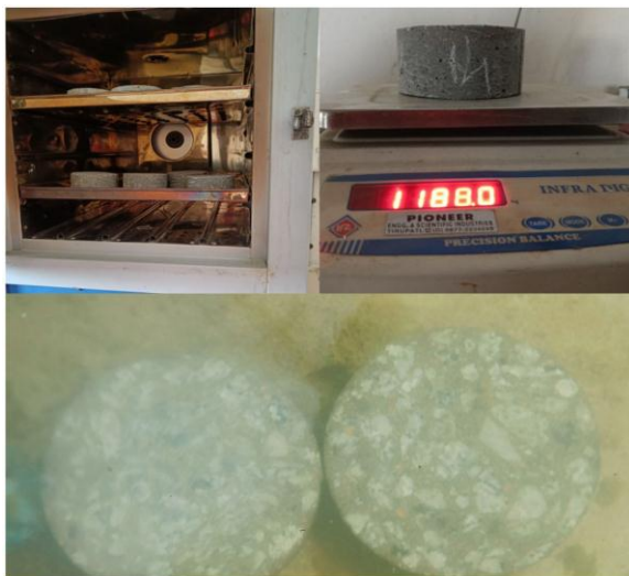
Fig: water absorption test
