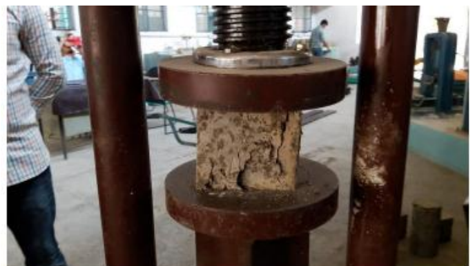
Figure 3.5 Cube compression strength test
