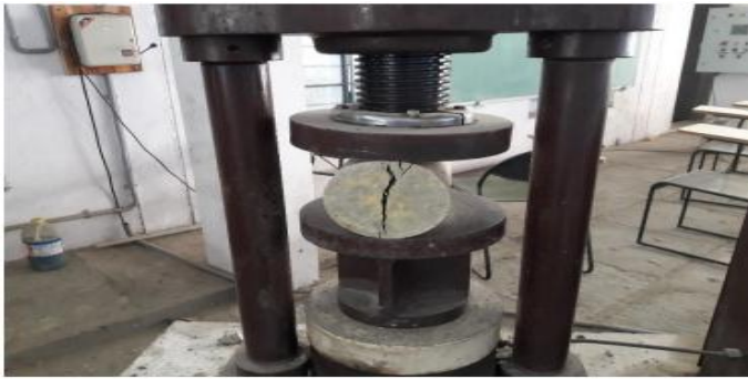
Figure 3.6 Cylinder split tensile strength test
