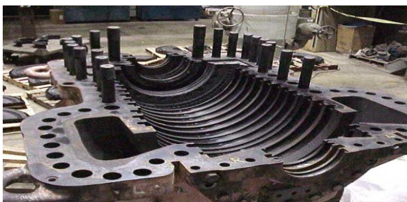
Fig-1.3 Steam Turbine Casing
