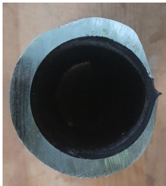
Figure 3.1 (c): Cross section at the failed region of RH tube.
