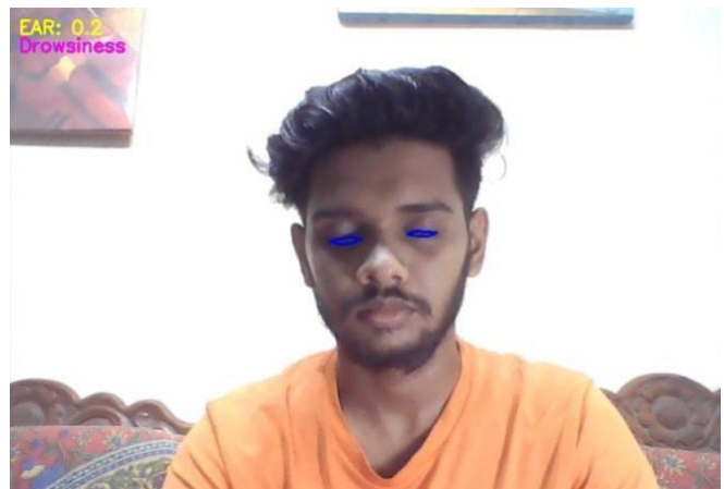
Fig-3: Drowsy eyes give a warning since an EAR is less than the threshold.
