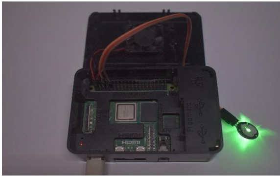
Fig-4: Raspberry Pi with PPG Sensor
