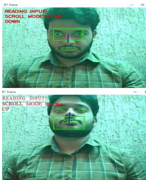
Fig 7.4 Illustrates the action of Squinting of eyes to turn on the scrolling mode on and down, up scroll movements of cursor.
