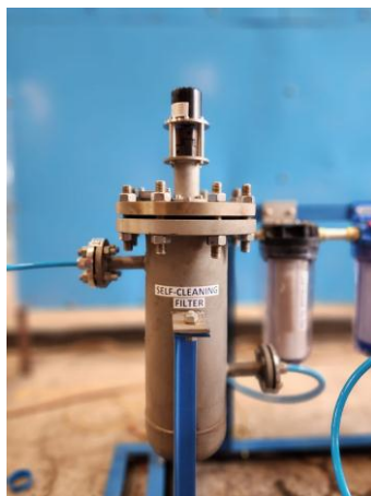
Fig-4: Automatic Self-Cleaning Strainer
