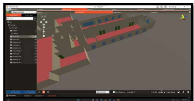
Fig 6. Building model generation
