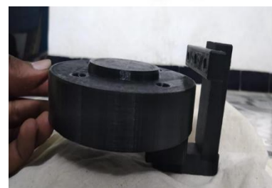
Fig -1: SMED designed model jig and manufacturing of nylon jig (3D printing)
