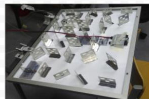
Figure 15: Second approach Randomly oriented fins arrangement
