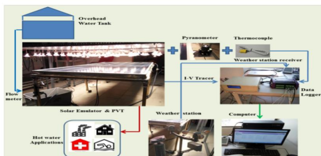
Figure 10: Schematic of Experimental Setup ( H. Fayaz et al. 2019)
