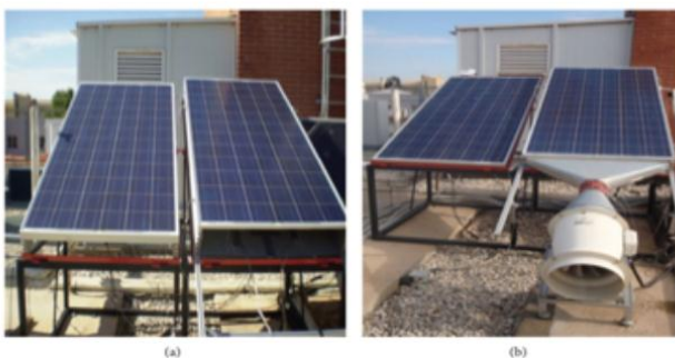
Figure 1: Experimental Setup (Y.Tripanagnostopoulos et. al.(2017) ) Left panel is a reference & Right panel is above a steel plate, creating an air channel underneath it. a) First setup Natural convection b) Second setup Forced convection
