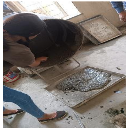
Fig 2: flowability test (Concrete Pouring)
