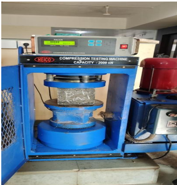
Fig 4. Compressive strength test
