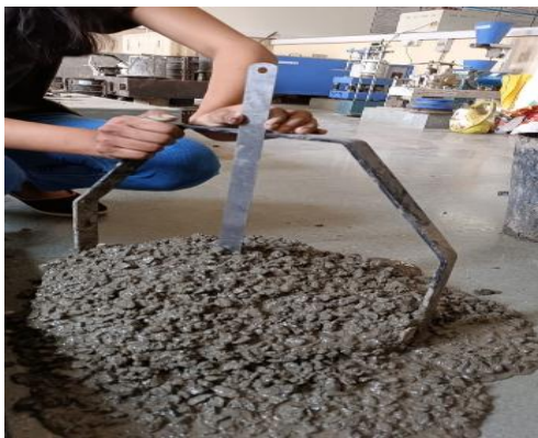
Fig 1: flowability test (Concrete Pouring)
