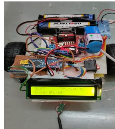
Fig-5: Charging of Battery using Magnetic coil
