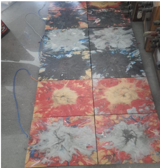
Piezoelectric plastic tiles arrangement
