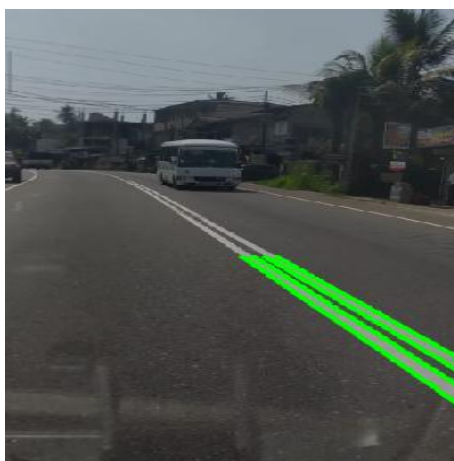
Fig-8: Road Lane Line detection in our research
