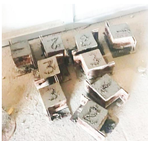
Fig -3.1: Cube Moulds for finding Compressive strength
