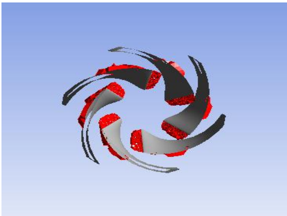
Fig.3.6 Stimulation Result of Cavitation Analysis showing cavitation-affected regions in red.
