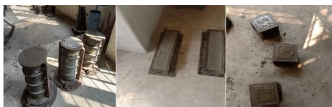
Fig 3: Cubes, beams and cylinders
