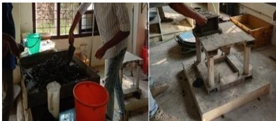
Fig 2 : Mixing and compaction of specimens
