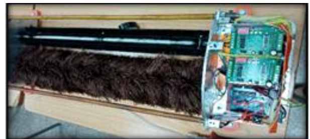
Fig -2: Selected design for PV cleaning system
