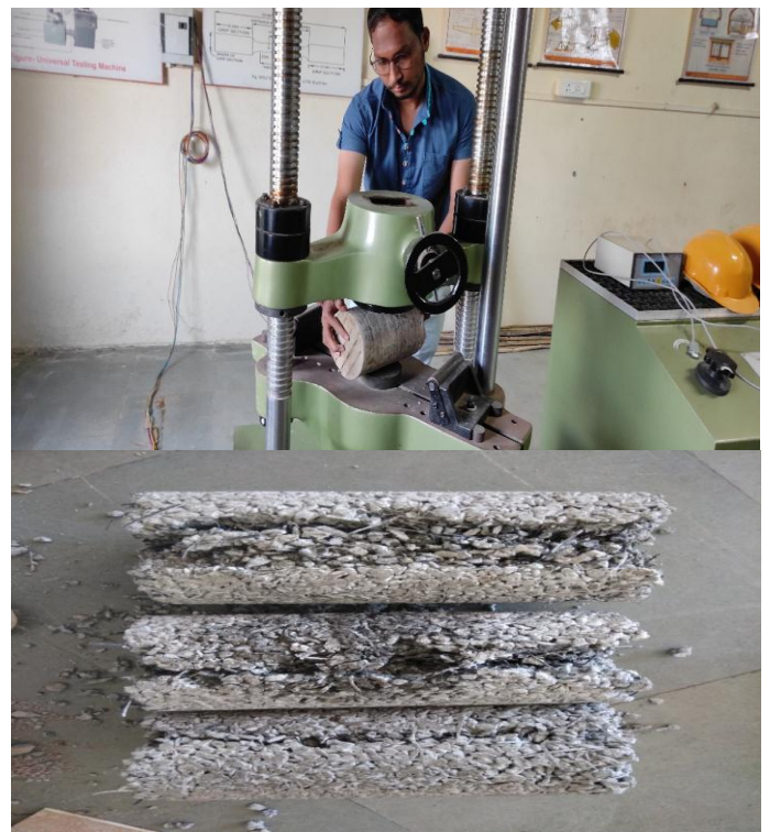
Fig. 4 Split tensile strength test
