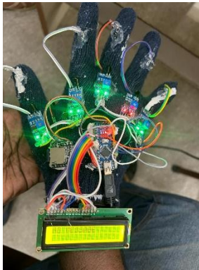
Fig-2: Working model of smart speaking glove using IR sensor
