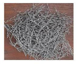
Fig -2: Steel fibres
