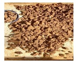
Fig -1: Drinking water treatment sludge
