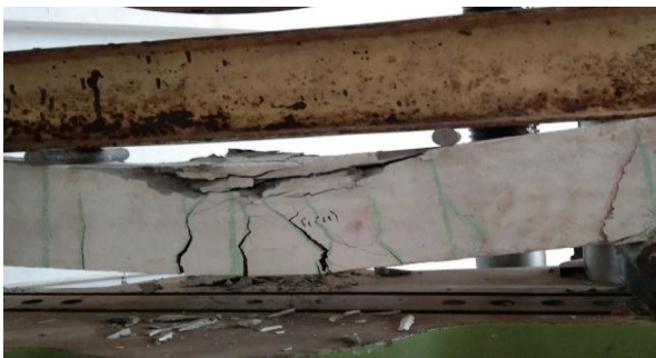
Fig-8: Flexural crack formed in the observed specimen at failure load.
