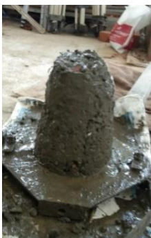
Fig- 4: Slump obtained at 0.25 % MPW fibre dosage
