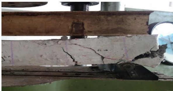
Fig -10: Shear crack formed in the MPW fibre reinforced specimen
