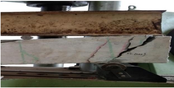
Fig-9: Shear crack formed in the control specimen.
