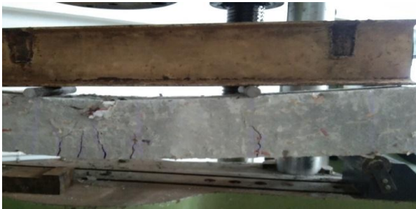
Fig-7: Flexural crack formed in the MPW fibre reinforced beam at failure load.
