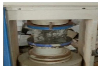
Fig -5: Fracture occurs in the cube at failure load
