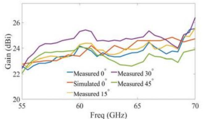
Figure-8: Gain was measured at a variety of beam angles, and simulated gain was also provided for the zero-degree beam.
