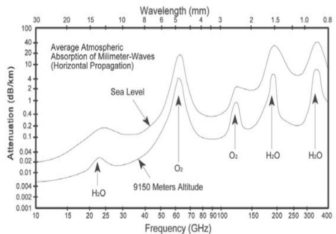
**Figure-2: Moisture vapor and oxygen absorption cause mm-wave attenuation**
