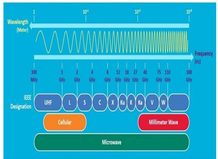
Figure-1: Millimeter-wave frequency bands.
