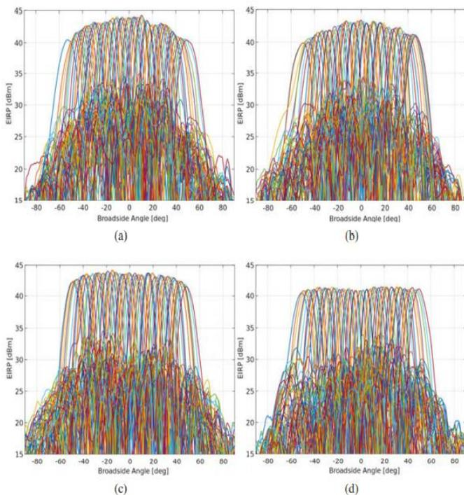
Figure-6: Antenna module supports four WiGig channels and 64 beam emission patterns. At 58.32, 60.48, 62.64, and 64.80 GHz, phase shifters have maximum gain and the signal chain is saturated.
