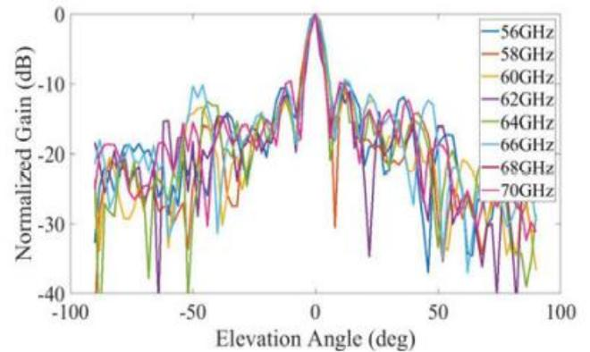
Figure-7: Radiation pattern at various frequencies between 56 GHz and 70 GHz, as measured in the elevation plane (E-plan).
