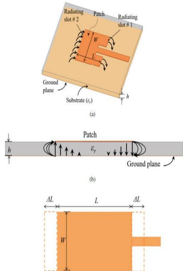
Figure-3: Microstrip patch antenna
