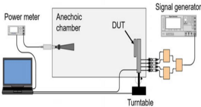
Figure-5: The measuring system used to create the TX beam book is shown in a block diagram.
