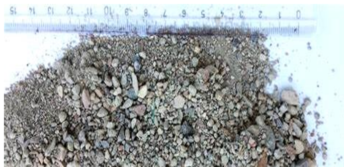
Fig -1: Demolished Fine aggregate
