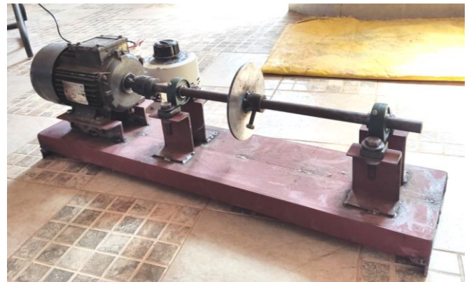
Fig. no-2: Bearing test Rig
