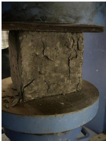
Fig-2: compressive strength test (N/mm 2 )
