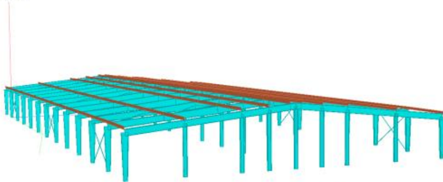
Fig 6- Render result of PEB structure using Staad Pro
