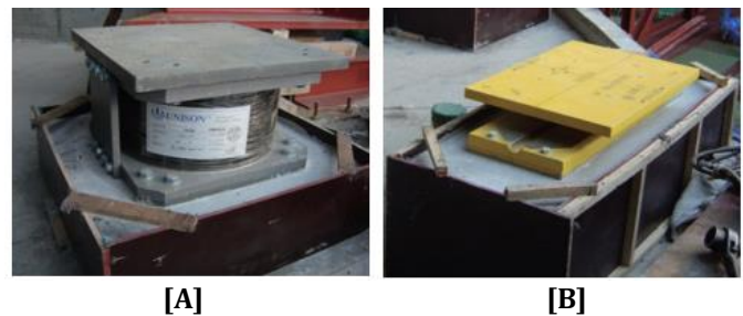
Fig. 4: - Bearings used in this study: (a) lead rubber bearing; (b) linear motion bearing [4]
