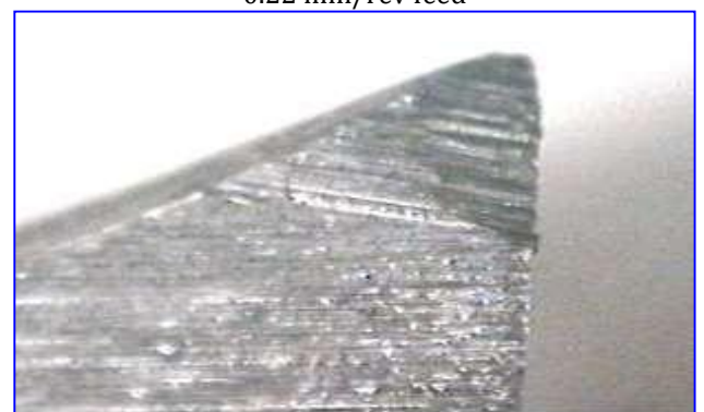
Fig. 4.11 Micrograph shows Flank Wear at 295 rpm and 0.45 mm/rev feed
