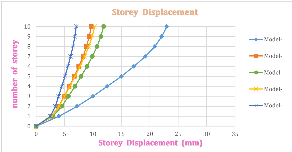
Chart 5: Variation of storey displacement for HDRB base condition and types of bracing.
