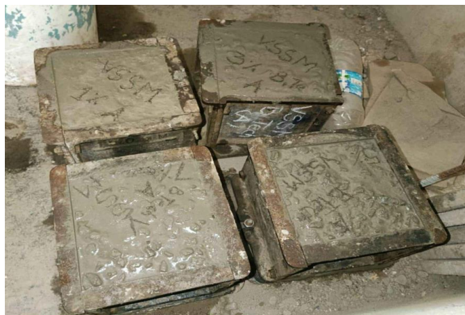
Fig. 1 - Casted concrete blocks
