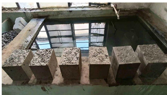
Fig. 2 - Curing of casted blocks in water tank
