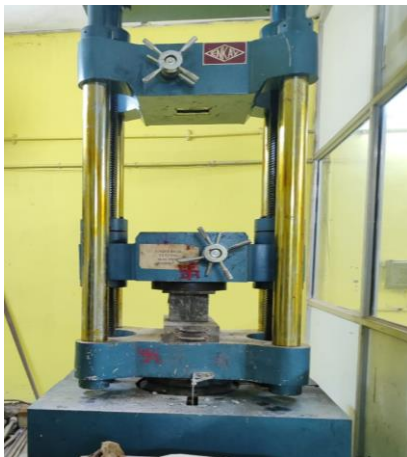
Fig-3: Compressive strength-test of concrete cube in U.T.M.
