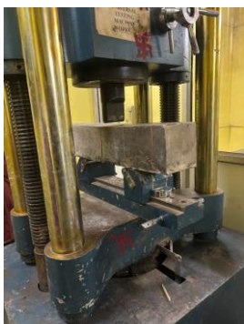
Fig-: flexural strength test in U.T.M.
