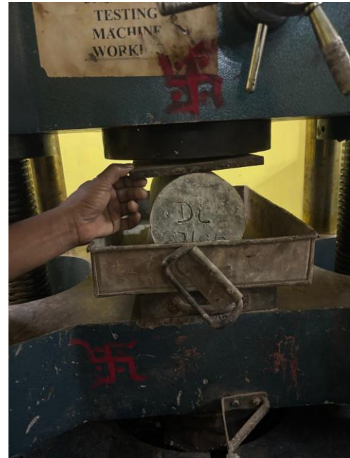
Fig-4: Split tensile strength-test of cylinder in U.T.M.
