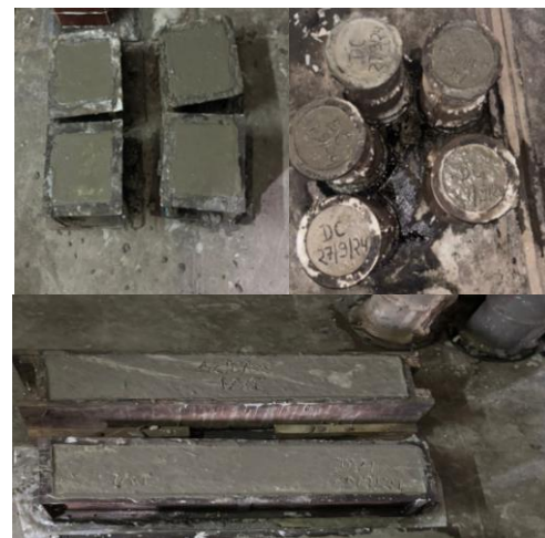
Fig-2: - Casting of Cubes, Cylinders & Beams.
