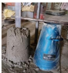
Fig 1 Slump cone test of concrete
