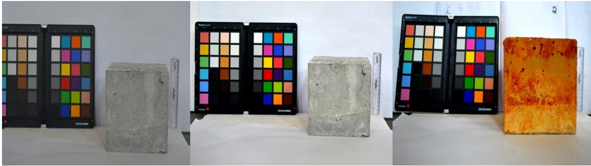
Figure 1. (a) Uncalibrated control sample; (b) calibrated undamaged control sample; (c) calibrated damaged Sample
