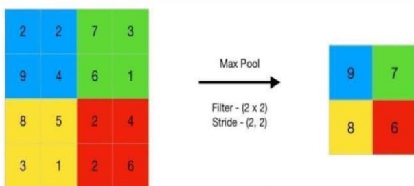
Figure 5.1 Max Pooling Layer
