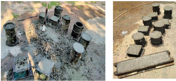
Fig-01 Casting process of concrete for beam cube and cylinder
