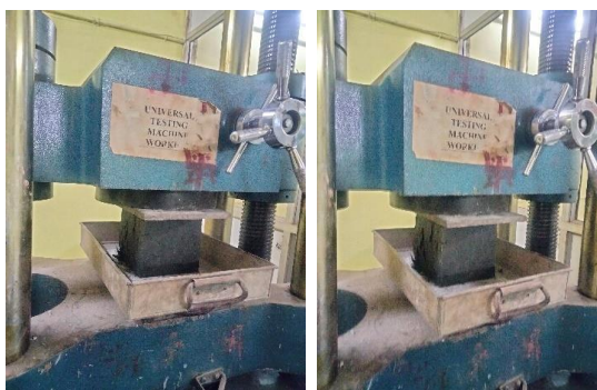
Fig -02 Compressive strength test of concrete cube in UTM
