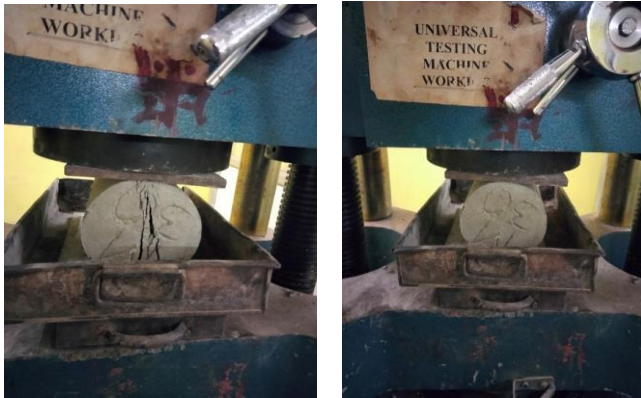
Fig- 03 Split tensile strength test for cylinder.
