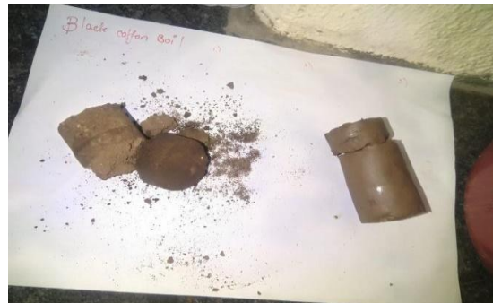
Fig. 5 Unconfined Compression Test of Soil
