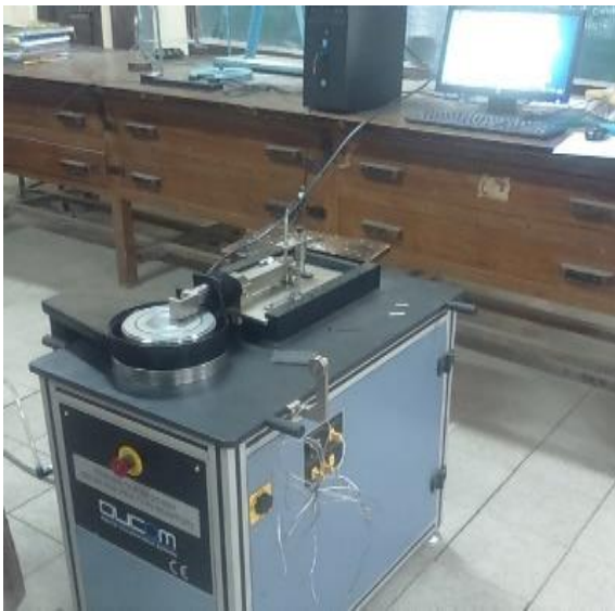
Figure 4: Experimental setup for wear and friction tester
