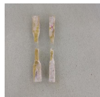
Figure 3.2: Specimens after tensile test components
