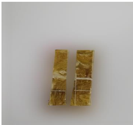
Figure 3.3: Specimens before impact test
