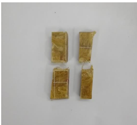
Figure 3.4: Specimens after impact test
