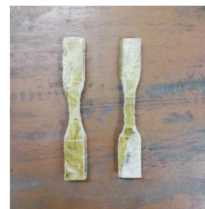
Figure 3.1: Specimens before tensile test
