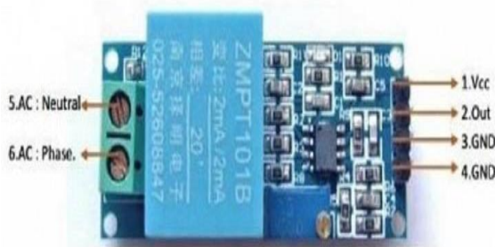
Fig-4: Pin diagram of voltage sensor (ZMPT101B)
